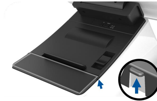
Figure 5. In case of paper jam, exert upward pressure on side rib (blue arrow) to open paper jam printer door (light gray)
