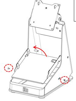
**1**- Remove (2) screws (L & R side) and pull out printer tray. Keep screws for reassembly.
