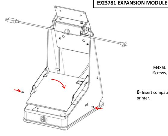
**4**- Re-assemble printer tray using (2) screws, L & R side.
