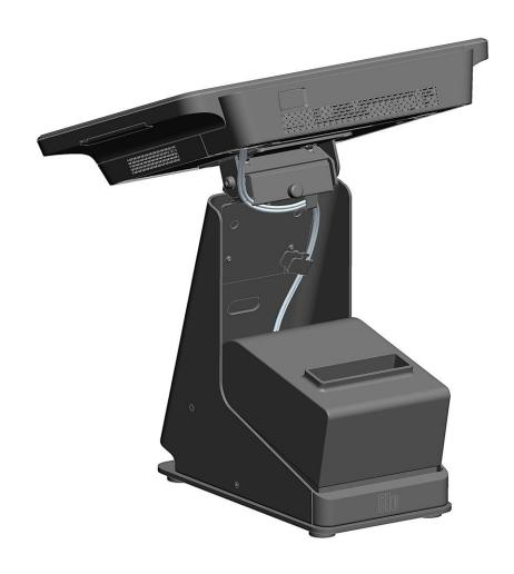
$oldsymbol{3}$  Attach cables to printer and place into stand.
