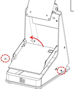
**1**- Remove (2) screws (L & R side) and pull out printer tray. Keep screws for reassembly.
