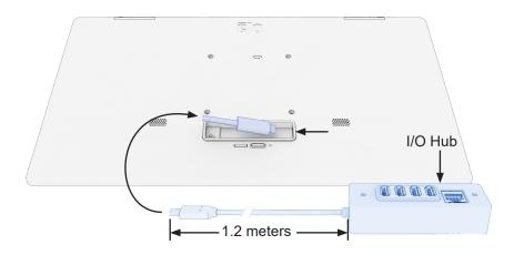
**3** Reinstall the cable locking screw and bracket on the rear of the I-Series 4 Slate display. The bracket slides in at an angle and has two small hooks that engage with slots inside the cable cavity. The bracket must be secured with the included screw.
