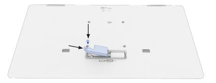
4 Secure the USB-C cable on the back of the I-Series 4 Slate display with the cable security bracket. The I/O hub has two threaded mounting holes which allow it to be mounted out of site. See dimensional drawing for mounting hole details.
