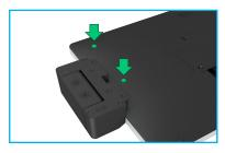
5.Remove the protective film from the included mylar covers and place the covers over the screws.
