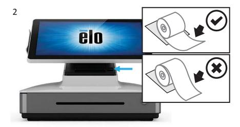
**Install receipt paper:** Install the paper by pressing the lid release button and lifting up the printer lid. Note the correct paper orientation from pictures above. **Do not use paper that exceeds 80 mm in width.**
