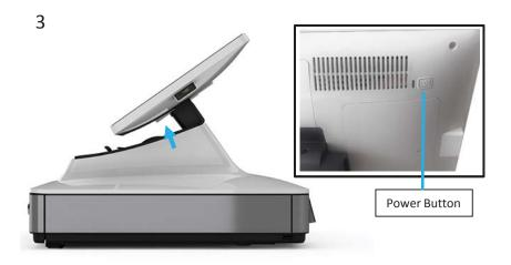
**Power on the register:** Press the power button (located on the back of the display head).
