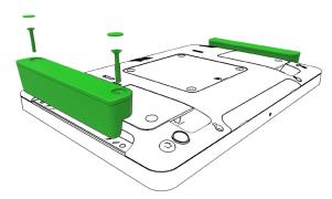
Gently press the status light into the Edge Connect peripheral bay making sure the connector is seated. Then install the included screws and screw covers.
