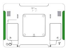
Remove the Edge Connect peripheral covers to expose the peripheral bay. Up to two status lights can be installed on a single I-Series display
