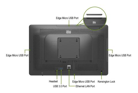
**3** Make additional connections from the bottom of the stand module or the Touchcomputer.
