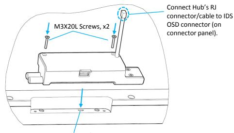
Remove the IDS accessory cover. Carefully align the micro-USB connectors. Secure the Collaboration Hub with (2) M3X20L screws.
